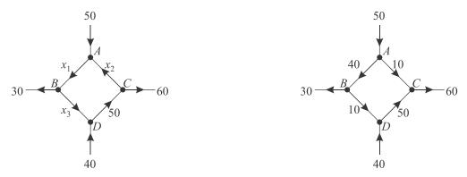
Network node Flow In Flow Out
