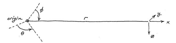
in other words,  $\Delta r \to \Delta x$ ,  $r \sin \phi \Delta \theta \to \Delta y$  and  $r\Delta \phi \to \Delta z$ . The mass continuity equation (1.10) can be expanded as:
