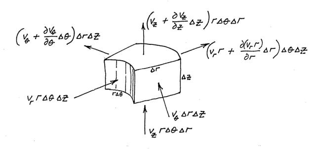
The term  $\partial M_{cv}/\partial t$  is zero because  $\rho$  is constant. Note also that the "in" arrows cancel, respectively, the leading terms of the "out" arrows. Dividing the three surviving terms by the control volume  $r\Delta\theta\Delta r\Delta z$ , we are left with
